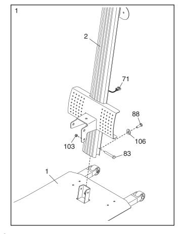
Insert the connector of the Lower Wire Harness
